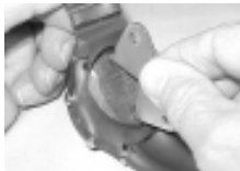
Fig. 113A - BATTERY HATCH REMOVAL (Tool)
