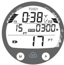
Fig. 58 - SAFETY STOP MAIN
