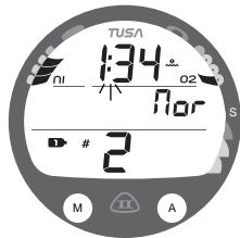
Fig. 12 - SURFACE MAIN (after dive 2)
