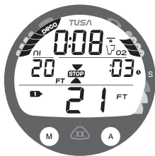
Fig. 60 - DECO STOP MAIN
