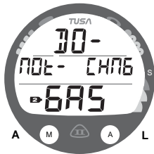
Fig. 70 - DO NOT CHANGE GAS ALARM
